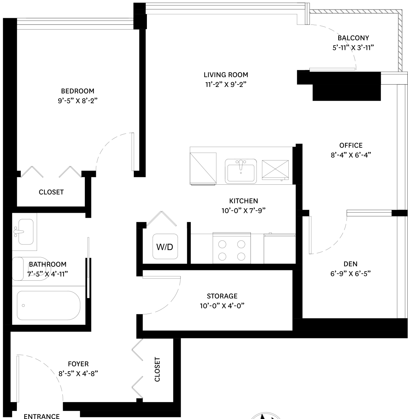
MAIN FLOOR PLAN Ceiling Height: 8'-0"
